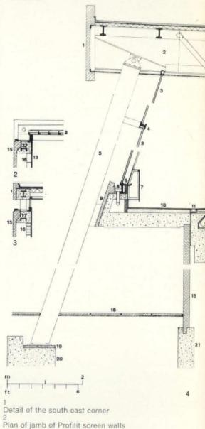
Section through slot window in screen wall
