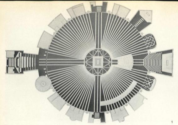
The design of the sanctuary floor, by David Atkins, echoes the sixteen concrete frames of the structure of the cathedral. From the edge of the sanctuary, lines of white marble radiate to the outer wall of the nave and the pattern extends into the Chapel of the Blessed Sacrament and the two towers on either side and into the Lady Chapel
