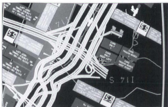
Computer image of a dynamic map from the Automatic Surveillance and Control System of the New Jersey Turnpike. Managers monitor traffic volume and flow interruptions from a central control point
