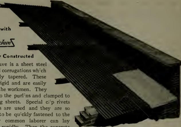
Ferroinclave is a sheet steel with dovetail corrugations which are inversally tapered. These sheets are rigid and are easily handled by the workmen. They are riveted to the purlins and clamped to the adjoining sheets. Special clip rivets and crossies are used and they are so designed as to be quickly fastened to the sheets. Any common laborer can lay these sheets rapidly. Then the concrete is applied to the upper and lower sides of the Ferroinclave without the use of forms.
