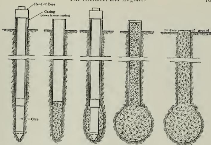
SHOWING METHOD OF FORMING PEDESTAL PILE
