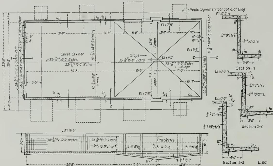
FIG. 5.—PLAN, LONGITUDINAL ELEVATION AND PARTIAL SECTIONS OF SWIMMING POOL IN CHICAGO HEBREW INSTITUTE
