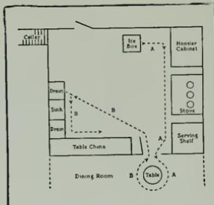
Floor plan of Applecroft Experiment Kitchen properly arranged and equipped. Notice saving of steps and time both in preparing and clearing away a meal. a. Preparing. b. Clearing away.
