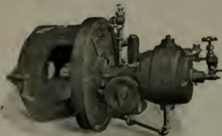
Improvements: Enclosed motors, dust, oil and water proof; oil-cooled motor runs 75 per cent cooler; oil heated electrically. Only one place to lubricate for entire machine, and many more exclusive features. Send for catalogue.
