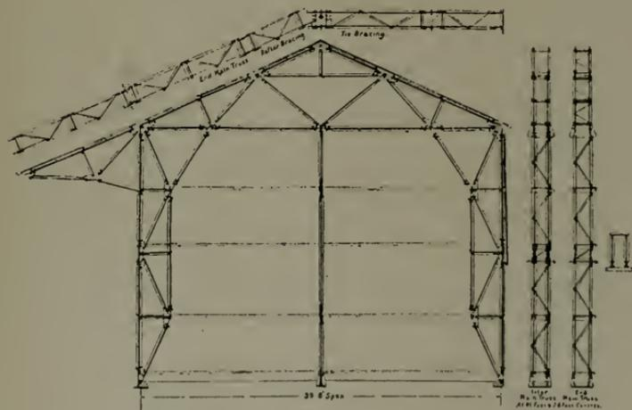
Fig. 2.—Cross Section of a Building Erected with Standard Steel Units
