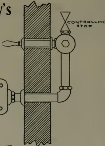
IS ESPECIALLY SUITABLE TO SCHOOL, HOSPITAL, COMFORT-STATION AND INSTITUTIONAL installations where utility chambers are available and vandal-proof equipment is desirable. Of rugged construction in finest bronze. Adapted for use on any water-pressure above five pounds — direct or indirect; cannot be held open to waste water and require no regulation for variable working conditions.
