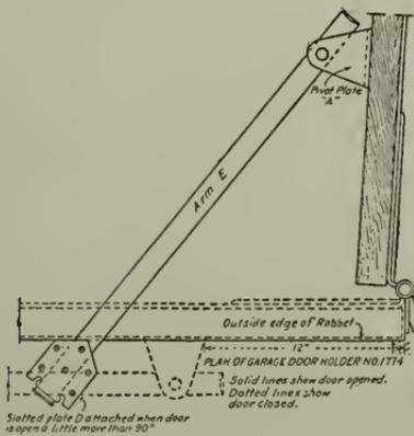
THE importance of avoiding possible damage and injury due to a swinging garage door is so well understood these days that swinging doors on new garages as well as old ones are now largely equipped with the Stanley Garage Door Holder No. 1774, which is recognized as being ideal for the purpose for which it is designed.
