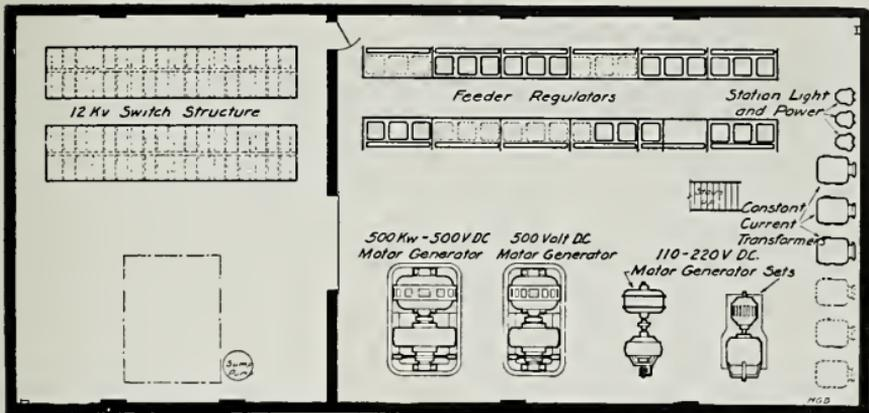
PLAN OF BASEMENT, SUB-STATION C., SAN DIEGO CONSOLIDATED GAS AND ELECTRIC CO.
