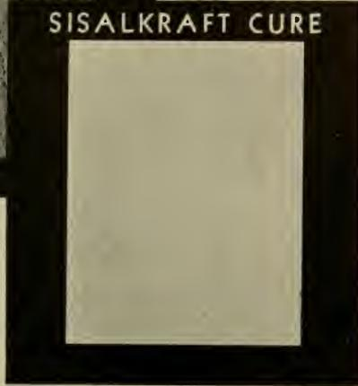
Proper curing made the difference in these two samples of concrete. Both were poured from the same mix. One received the usual air cure — the other was kept covered with the waterproof paper, Sisalkraft. Both were given the same accelerated wear test.
