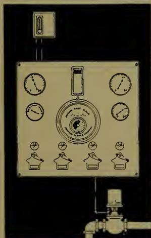
The illustration suggests Johnson apparatus for a typical Zone Control System. Control panel applies to a building having four zones. Zone control valve and dual type thermostat for day and night operation are indicated for one of the zones.
