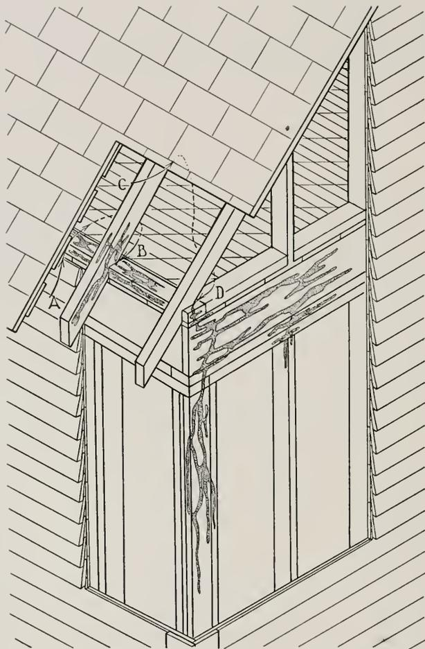
Fig. 10—Diagrammatic sketch showing workings of two colonies of the common dry-wood termite, *Kalotermes minor*, based on numerous observations of colonies in houses. The lines AB and CD mark the assumed original routes of entry of the two colonizing pairs. The galleries of the two colonies are not connected with each other.
