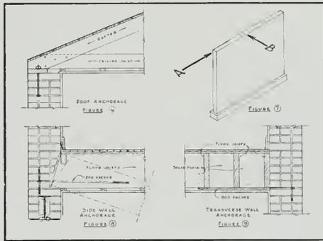
These connections are not only inadequate for transmitting diaphragm reactions into the walls but are likewise unsatisfactory for staying the walls against transverse displacement. This latter defect will be discussed in some detail later.
