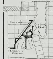
A heavy metal form built to proper angles and dimensions with a friction poker controlled damper which forms a perfect throat and down draft shelf. Prevents wrong construction and smoky fireplaces. Damper is easily adjusted, doubling heating efficiency, and should be completely closed when fireplace is not in use.
