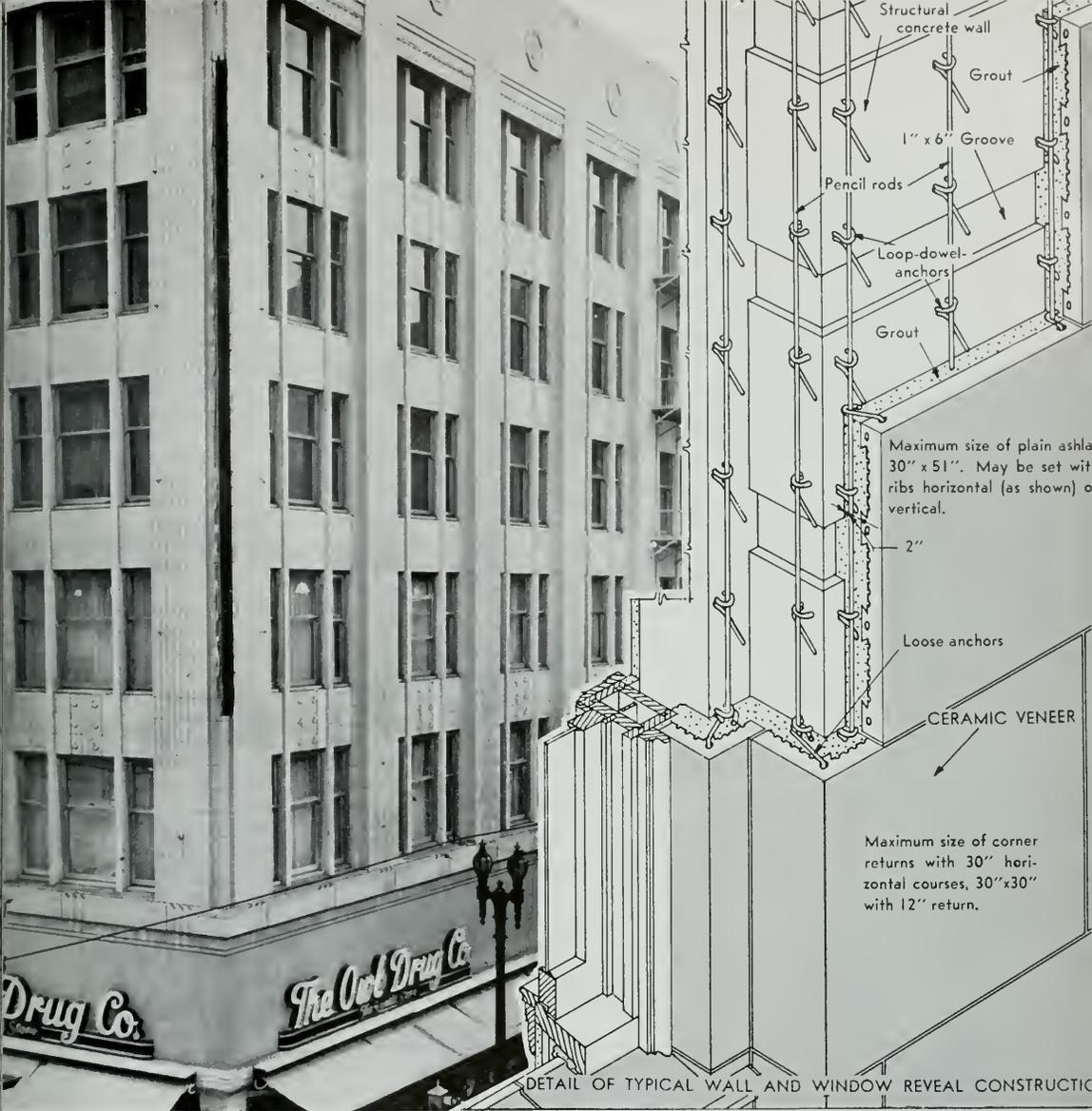
DETAIL OF TYPICAL WALL AND WINDOW REVEAL CONSTRUCTION
