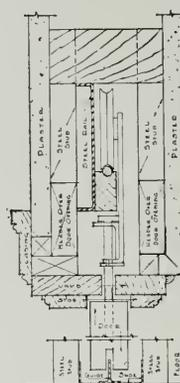
Joins with a 4" stud wall... steel studs... adjustable steel and wood track. Can be used for screen doors in connection with French doors; also to close arches. Send for detail drawing
