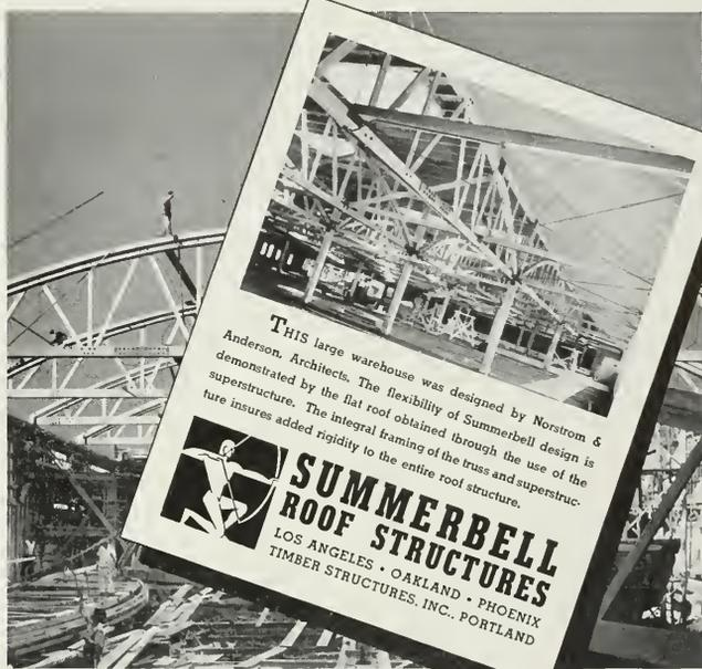
THIS large warehouse was designed by Norstrom & Anderson, Architects. The flexibility of Summerbell design is demonstrated by the flat roof obtained through the use of the superstructure. The integral framing of the truss and superstructure insures added rigidity to the entire roof structure.
