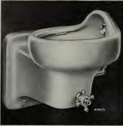
**HAWS Model No. 7A** . . . vitreous china wall drinking fountain with bubbler protecting cowl . . . chrome-plated brass raised anti-squirt angle stream head with self-closing automatic stream control valve . . . all working parts accessible without detaching unit from wall.
