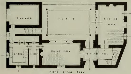
**LEFT:** First and second floor plan. The finished work closed the outside wall of the patio up to the level of the second floor gallery, and a door from the garage opens into the patio.
