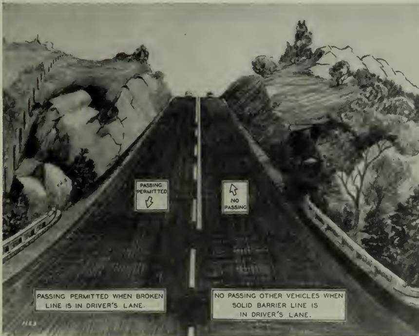
**"NO PASSING" Yellow Line Doomed: The YELLOW traffic line on California's State highways is being replaced by the uniform National system of highway signs and traffic control devices—two continuous parallel white lines where passing a vehicle is prohibited, and a combination solid white line where passing is permitted IF the broken line is in the driver's lane.**
