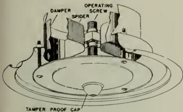
The cylindrical damper is raised or lowered by turning the extended shank of the operating screw. Any air volume may thus be quickly and easily obtained. Complete handbook available by writing manufacturer.
