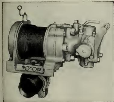
Capable of lifting 500 lbs., the "AIR WINCH" AW-80 weighs only 85 pounds, has a rope capacity of 150 feet of 1/4-in. rope, is 18 inches long, 9 1/2 inches high and 11 inches wide. It is powered with a four-cylinder, reversible, piston type air motor. Can be mounted in any position. Complete information Bulletin No. 76-H.
