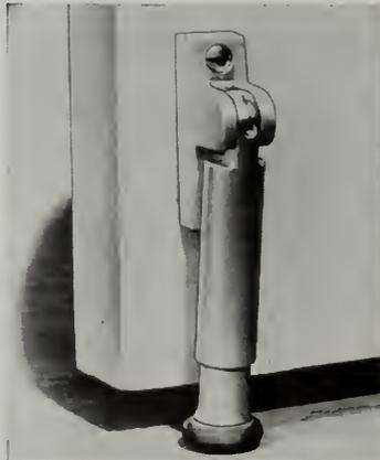
Employing the spring idea the "Doormaster" holds the heaviest doors without slipping. It is made of durable aluminum and mounts a tough rubber foot firmly to the spring loaded piston, and may be easily raised when not in use.
