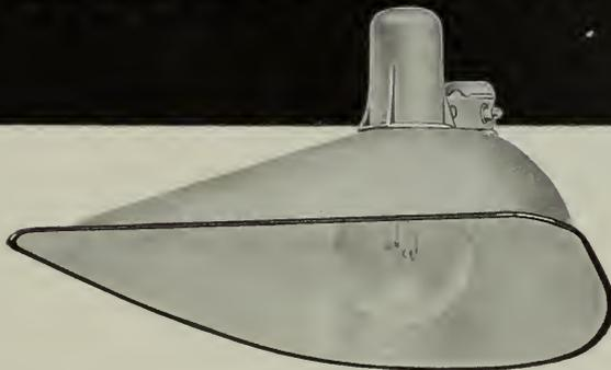
A highly efficient floodlight for use in service stations, parking lots, yards and other areas where maximum spread of light is desired. Finished in porcelain enamel, with neutral gray exterior. Supplied with mountings for wood cross-arms, 1" to 1½" pipe cross-arm or slip-over 1½" pipe mast. Takes 750/1000/1500 W. lamp.
