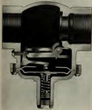
Easily installed in gas or oil supply lines for industrial furnaces, institutional heating plants, public utility supply systems, the new Warden Valve (manufactured by the Security Valve Company of Los Angeles) is available in sizes 1½" to 8" diameter.
