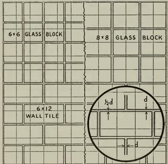
**THE MORTAR JOINT** is automatically provided for with modular-coordinated units. Net size plus standard mortar joint (d) equals nominal size, thus the architect need work only with nominal dimensions.
