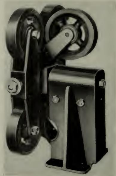
The Elsco Roller Guide contacts the guide rail with rollers mounted on compensating arms designed to yield automatically under varying conditions of use and yet to maintain constant contact with the rail. Elimination of friction results in savings in maintenance and current, and eliminates greasing of the rails with a consequent reduction of the fire hazard in the shaftway.
