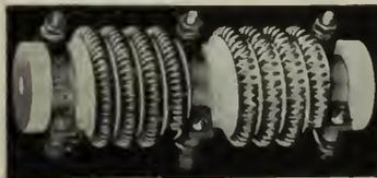
Center and end taps are half-straps securely clamped to the core, assuring absolute mechanical rigidity independent of support by the resistance element. Brass nuts and bolts and stainless steel lock washers are used, with all parts zinc plated.
