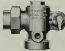
An exclusive feature of the valve is the opening provided beneath the seat to direct the air and gases to the Thrush Pressure Tank before they are circulated in the system, thus permitting the selection of as many different temperature zones as are required.
