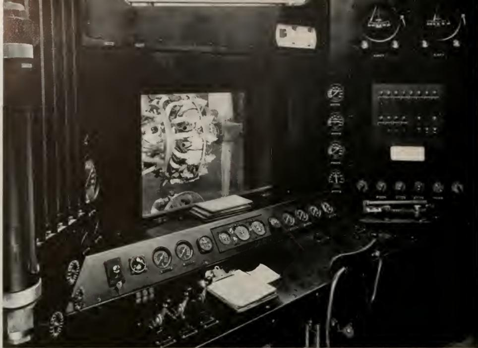
All of the operating controls and metering devices required for engine testing in the new "test cells," are grouped around double-glazed observation windows in compact and convenient arrangement. Six control desks, similar to one illustrated above, are paired in the control passages extending through the cell block. Sperry controls (left foreground) and potentiometer is mounted flush on desk at right with slant gauge directly above window. Engine in position for testing is seen in test cell.
