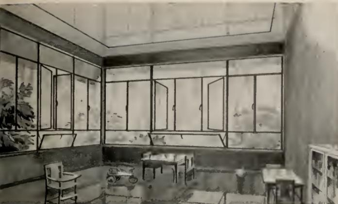
Fenecraft Combination Windows, Types 636 and 616, joined with steel mullions to provide abundant daylighting—ideal for a hospital nursery. Sill vent tilts in—guards against drafts, prevents children falling out.
