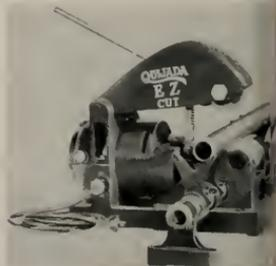
Manufactured by the Quijada Tool Company of Los Angeles, California, this portable machine has an integrally-mounted 1/2 h.p. 110-volt, universal type AC-1 motor with a direct gear drive the rollers. Gears are self lubricating. Automatic trip switch starts cutting operations when the cutting wheel contacts the pipe and automatically stops when the cutting is finished.
