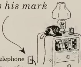
That built-in telephone outlet is the stamp of a careful builder. He added conduit and outlets while the home was under construction. The cost was insignificant . . . just a few pieces of tubing leading to convenient telephone outlets provide raceways for telephone wire.
