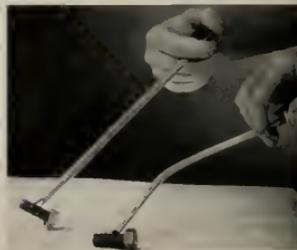
The shaft is flexible cable encased in flexible housing with expanding and retracting fingers which enable it to reach in and grab a tight hold on anything, with ample flexibility to work around corners or S-turns.
