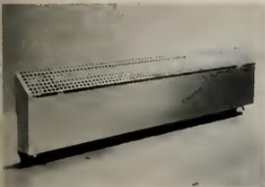
Equipped with built-in thermostat, pressure type fan with long life ball bearing motor the heater is available in 2, 3, 4 and 5 kw. for 236-volt a.c. operation. It is finished in smooth silver gray hammettone, or in neutral prime coat.
