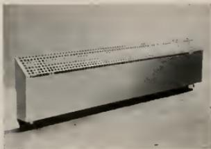
Requiring a minimum of space, it is easily installed and permits persons to work close to windows in comfort. Two steel tube circuits pass through fins giving maximum heat transfer to full area of 3" wide by 6" high fins. Made in sizes from 18" to 116" in length; height 8", and depth 3".
