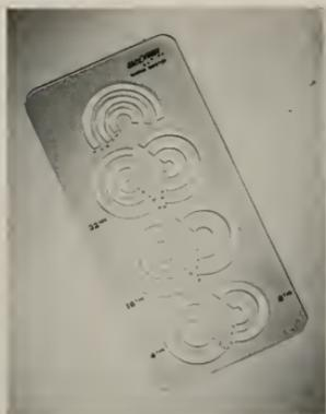
All edges are smooth and clean. Radius point is precisely located, the center hole serving the particular radius. Radii on inner contours run up to 37/32nds in 32nd increments.
