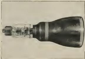
The new 7" tube is designed for use in dual-channel oscilloscopes having high sensitivity. Electric-static focus and deflection as well as adequate shielding against cross talk is used. Tube is normally coated with P1 phosphor, but other standard phosphors supplied upon request.
