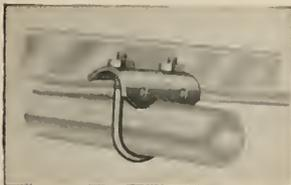
The Spedon retains a constantly effective clamping tension in the U-bolt provided by the saddle spring action, making it ideal for heavy-duty industrial applications. Bodies for 1 1/4"-1 1/2" can use either size U-bolt. Each is furnished with zinc-coated U-bolt and nuts assembled ready for use; available 3/4" to 2" pipe sizes. Complete data Spedon Pipe Clamp Co., 33-51 60th Place, Woodside 77, N. Y.
