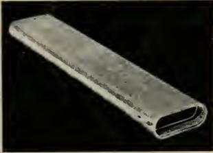
This new WV features an inner and outer pipe separated by an insulating air space; new "Fastloc" coupler enables pipe sections to be joined without cement or mastic, and without screws except where vent will be left exposed in rooms. Outer pipe is galvanized steel, aluminum is used for the inner pipe to provide fast heating inner "hot-stack" with maximum corrosion resistance. Manufactured by Metalbestos Division, William Wallace Co., Belmont, California.
