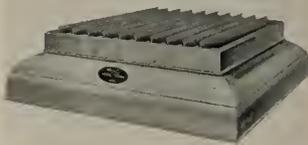
Completely functional, it is built entirely of heavy wall, extruded aluminum sections with all joints welded. Being of aluminum it is lightweight and can easily be installed by two men without need of special equipment. Requires no painting as it is impervious to rust and corrosion inside and out. Overall height is 21 inches, available in sizes 20" to 60", and in capacities from 3800 CFM to 42,000 CFM. Complete data from Iron Lung Ventilator Co., 5403 Prospect Ave., Cleveland 3, Ohio.
