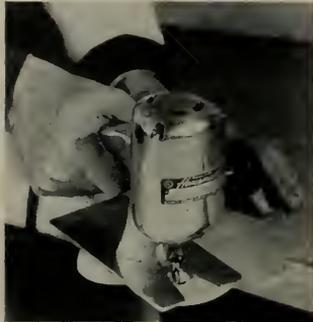
A rectangular base converts quickly for jig-saw work, while a circular base makes it a router—attached in an inverted position to a shaper table, the tool becomes a shaper and joiner in a matter of seconds; operated by powerful, AC-DC Universal motor; 40-page manual. For prices and literature, write PORTER-CABLE POWER TOOLS, Ltd., P.O. Box 1019, London, Ontario.
