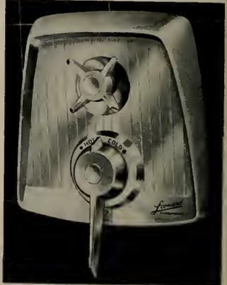
It automatically compensates for temperature and pressure changes in either hot or cold water supply. Selection of the desired volume, from soft-rain to full pressure will not effect resultant temperatures. Simple to install and maintain; no seats or seat packings in thermostatic housing; easily accessible check and stop valves. Mfg. Leonard Valve Co., 29 Laurel Ave., Providence 6, R. I.
