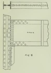
this force is. With a 45 deg. bracket the force 1/1 is just equal to the load 1/2, and diminishes as the angle between the seat and the bracket increases. These brackets are now usually made with a 60 deg. slope.
