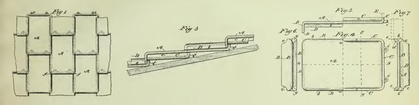
Fig. 1 is a plan view of several tiles arranged as they would be when laid upon a roof; Fig. 3, an enlarged vertical section taken on a line corresponding with xx in Fig. 4; Fig. 4, a plan view of a single tile drawn on the same scale as Fig. 3; Fig. 5, a sectional view of Fig. 4 at xx; Fig. 6 is an elevation of the lower end of the tile in Fig. 4; Fig. 7 is a cross section at yy of Fig. 4.
