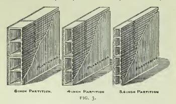
there to-day. The length of any one straight section of a partition is a more important element than its height, and judgment must be used in every case. I have built a 3 in. partition around two sides of an elevator shaft, 120 ft. high on girders in the cellar, the tiles being set on end; the weight at the bottom course was about 1,500 lbs. per lineal foot. This was only 94 lbs. per square inch of tile area.
