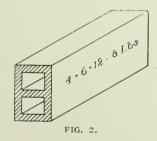
ends to hold the mortar joint. They, however, show the holes at the angles of partitions which have to be filled with mortar. Hollow partition tiles may now be had for partitions 2, 3, 4, 5, 6, and 8 ins. thick, and 12 in. partitions may be had by setting 6 by 12 in. tiles on the flat side. This is a handy way to build light fire proof vaults in buildings where there are sufficient foundations.
