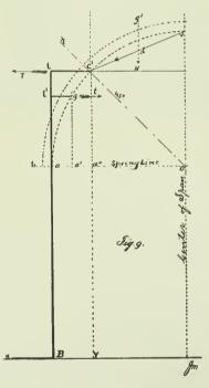
having the weight concentrated at the end B, then becomes the counterfort and balances the thrust—always assuming the pier is sufficiently rigid to sustain the load.
