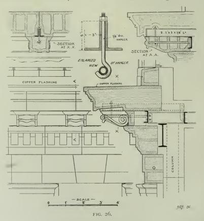
a cornice of much greater weight and projection to deal with, the same considerations hold good. The projection in this case is 3 ft. 6 ins., with 1 ft. inside the wall line. The modillions are spaced,
