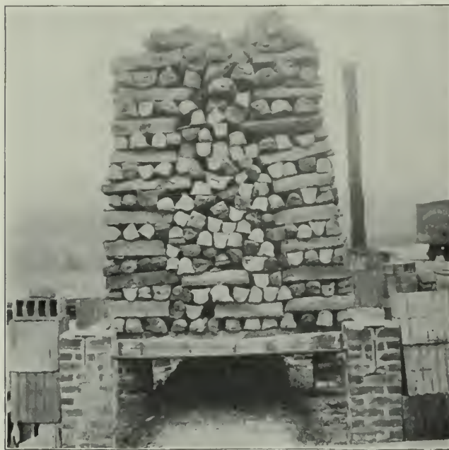
"NEW YORK" REINFORCED TERRA-COTTA ARCH. SIX-INCH END CONSTRUCTION BLOCKS—DOUBLE TRUSS, CARRYING SIXTEEN HUNDRED POUNDS PER SQUARE FOOT ON SIX-FOOT SPAN BY FIVE FEET WIDE.
