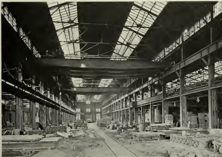
Example of Roof Lighting by Means of Flush Skylights
