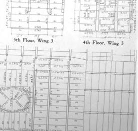
Third Floor Framing Plan Showing Bottom Chords of Trusses in Wings 3 and 4
