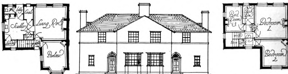
Half Floor Plans and Front Elevation, Cottage Houses for the Manchester Corporation
