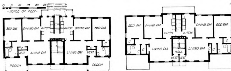
First and Second Floor Plans of Typical Four-Flat Houses
