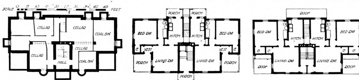
BASEMENT, FIRST AND SECOND FLOOR PLANS AND VIEW OF FOUR-FAMILY HOUSE OF ONE TYPE HOUSING DEVELOPMENT, BUCKMAN VILLAGE, CHESTER, PA.
