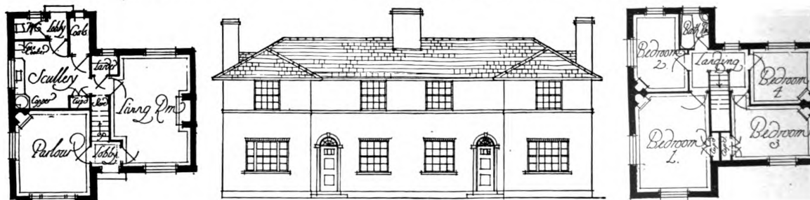
Half Floor Plans and Front Elevation, Cottage Houses for the Manchester Corporation Gordon Hemm, Architect
