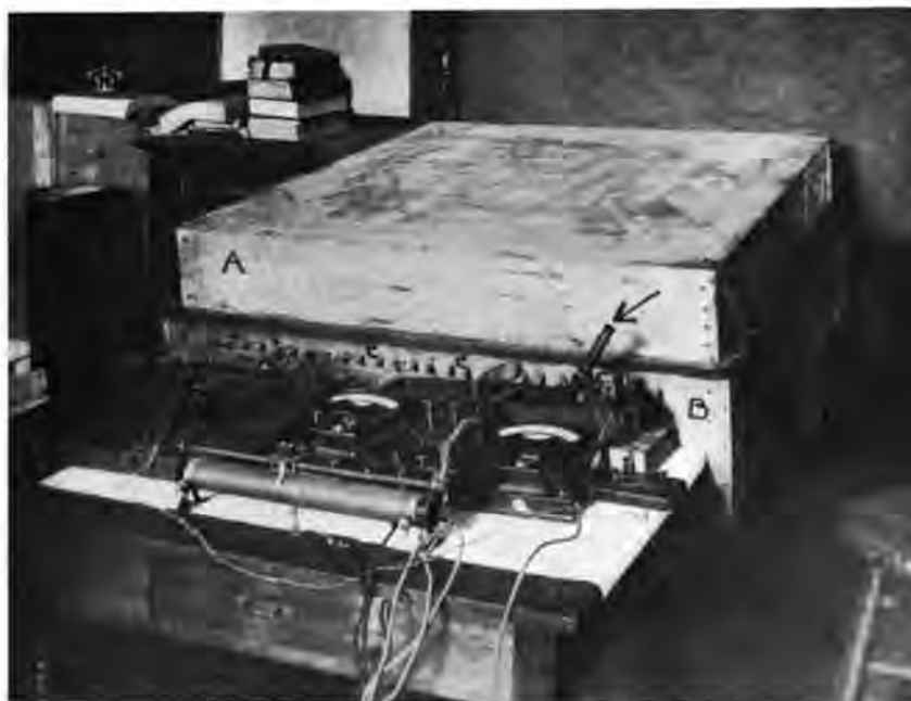
Fig. 1. Layout for thermal conductivity tests, showing sample (A) on insulated box (B), with electrical connections for thermo couples. Arrow points to reading microscope
