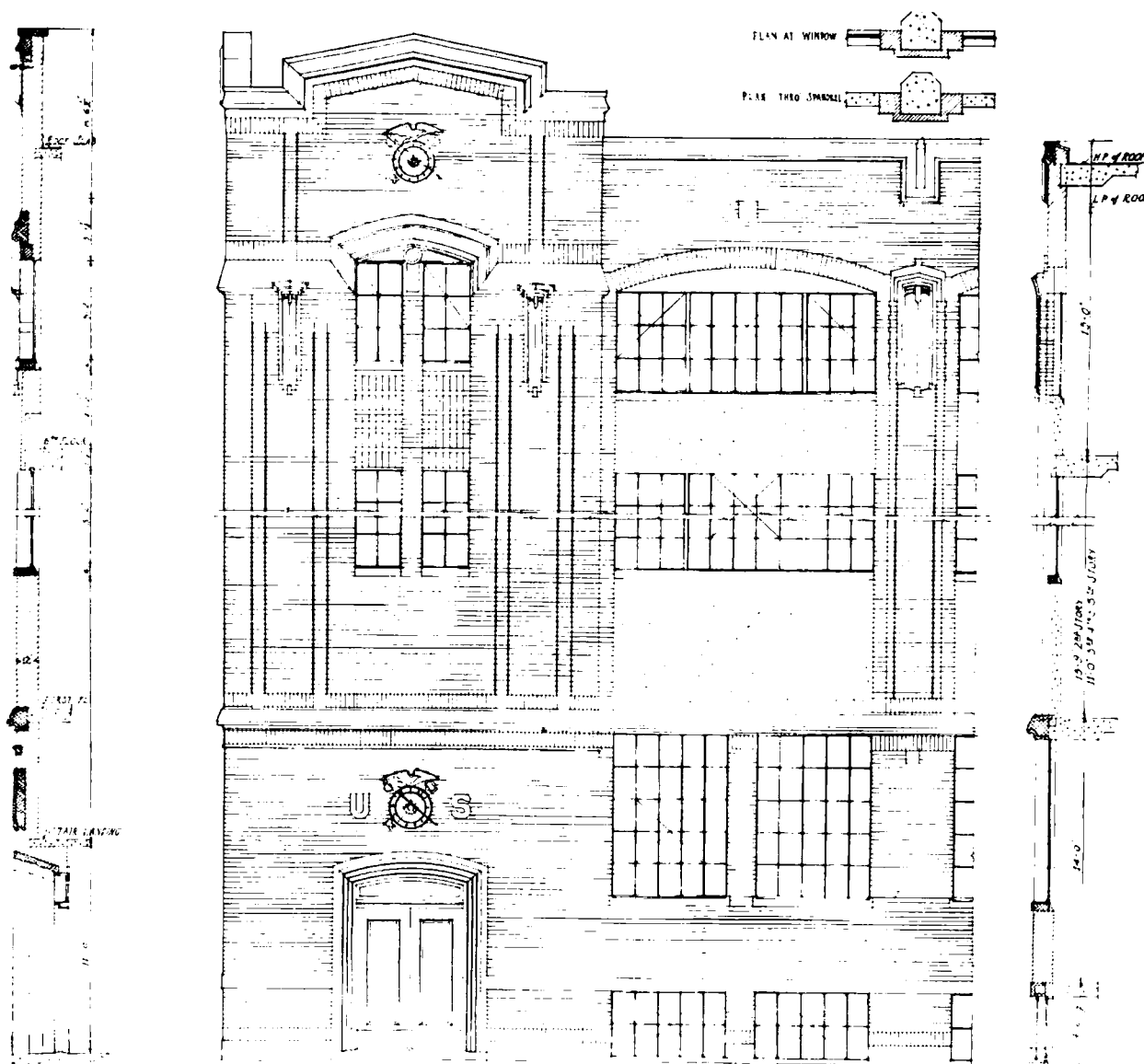
Wall Sections and Detail of End Bays. U. S. Army Supply Depot
