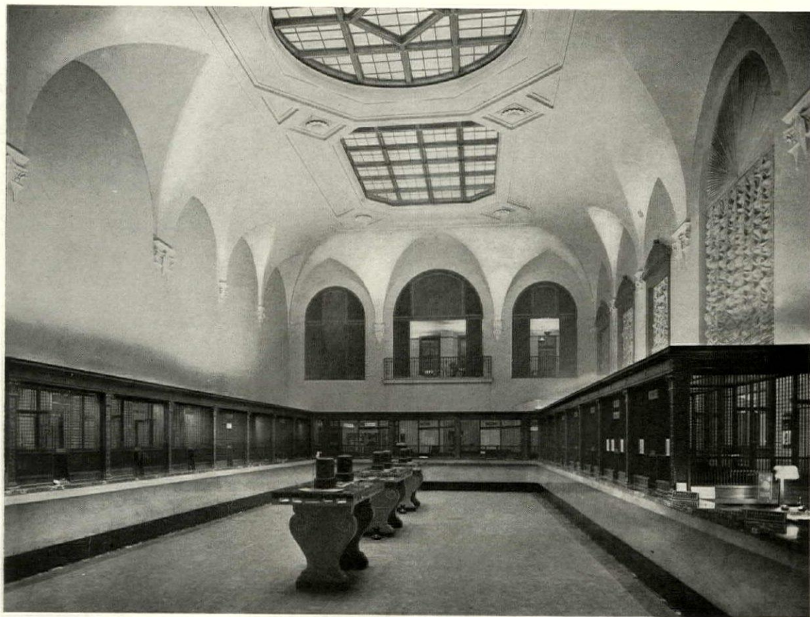
Fig. 3. 75-watt lamps in mirrored glass, direct lighting reflectors are used above the skylight; 100-watt lamps in inverted mirror reflectors above the cages provide indirect illumination and make the ceiling luminous
