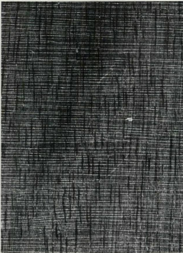
Cross Checks or Temperature Cracks
