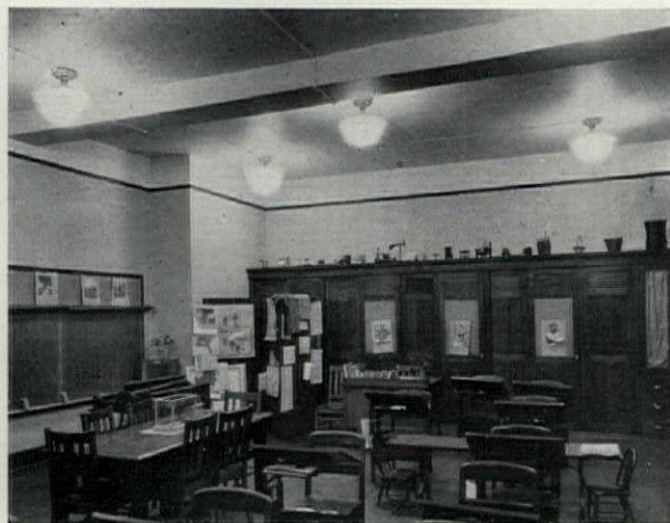
Room 24x30x13 Feet. Average Illumination of 15-Foot Candles Is Provided by Eight 300-Watt Lamps
