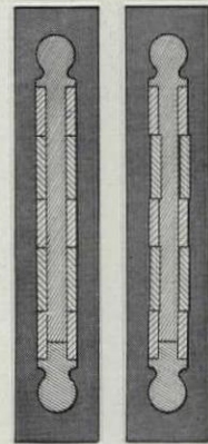
Illustrating the effect of lateral wear on the ordinary fixed pin. The moving knuckles bite into the pin like teeth. A sagging hinge is the result.
