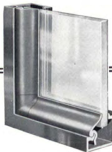
Section of Davis construction showing how the plate glass is safely held by the patented fulcrum principle, exclusively a Davis feature. The glass is set from the outside without the need for putty or plastic cement. Ventilation and drainage are afforded, if desired.
