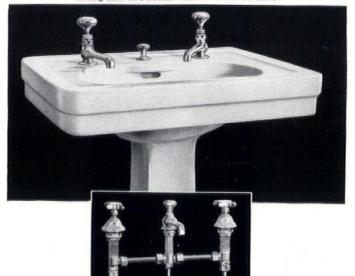
K-8002 Kohler Combination Lavatory Fitting, May be equipped interchangeably with compression valves as shown or with the self-closing type. This firtir ghas the positive-acting Kohler lift drain with patented spring ball to keep the drain open or closed.
