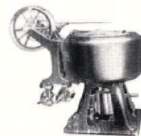
Marathon Extractor. Belt drive, with angle counter- shaft attached.
