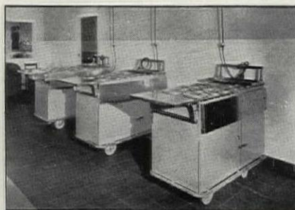
Some of the Ideal Food Conveyors with Monel Metal tops, covers and shelves in the Medical Center, manufactured by the SWARTSBAUGH MFG. Co. of Toledo, Ohio.
