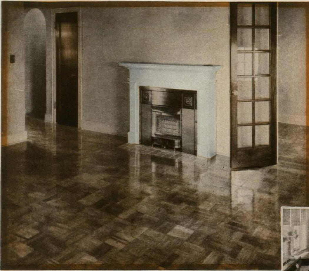
\*CELLized oak floor blocks are complete square units, in three sizes: 6 $\frac{3}{4}$ -in., 9-in., and 11 $\frac{1}{4}$ -in. squares—in all grades. Each block is full  $\frac{15}{16}$ " thickness, of 3 or more oak strips splined together. Side and end matched.
