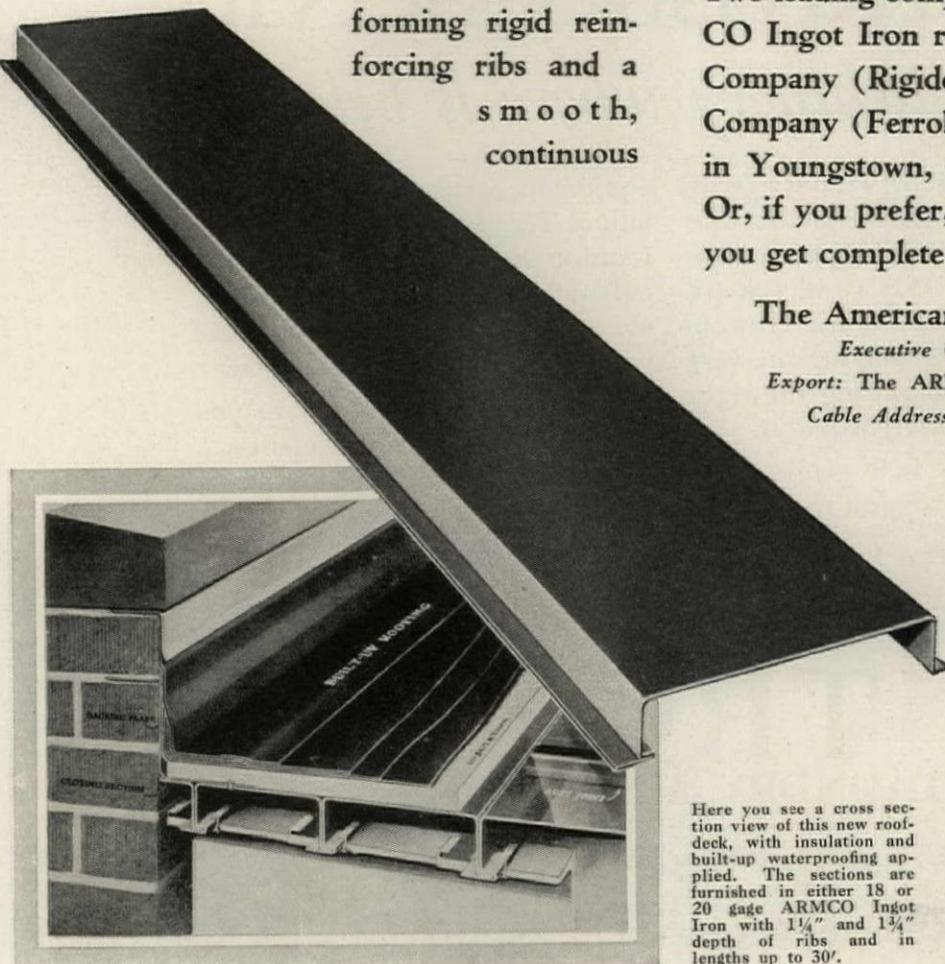
Here you see a cross section view of this new roofdeck, with insulation and built-up waterproofing applied. The sections are furnished in either 18 or 20 gage ARMCO Ingot Iron with  $1\frac{1}{4}$ " and  $1\frac{3}{4}$ " depth of ribs and in lengths up to 30'.
