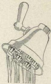
*A turn of the lever sluices all sediment away.*
