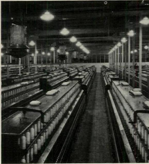
Textile mill. Spinning. 300-watt clear lamps, diffusing globes. Outlets spaced 14 x 21'. Lamps 12' above floor, ceiling 14'. Ceiling white, walls principally glass. Illumination level 8-foot-candles.
