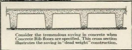
Consider the tremendous saving in concrete when Concrete Rib floors are specified. This cross section illustrates the saving in "dead weight" construction.
