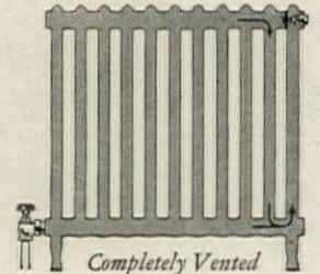
IN-AIRIDS located within the radiator cannot be tampered with. Their invisibility also adds to the appearance of the radiator.
