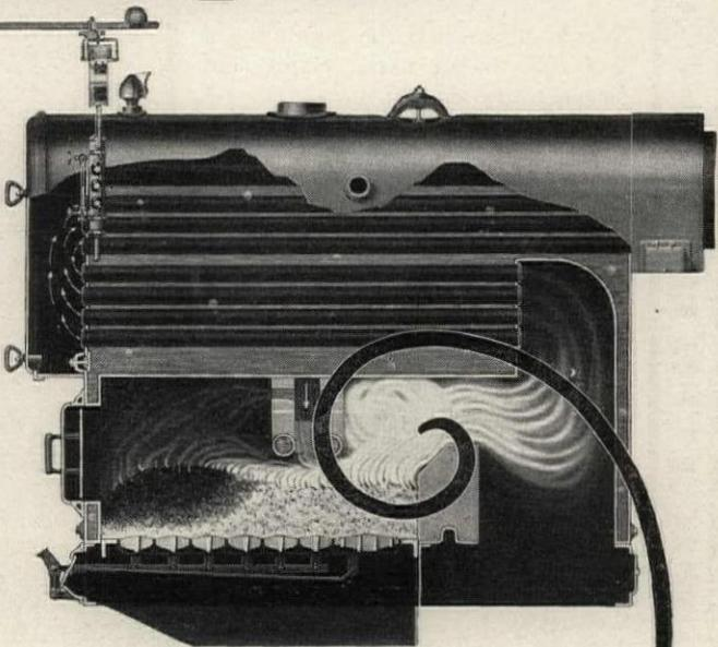
additional oxygen but thoroughly heats it before passing it down onto the fire. A refractory bridge wall to the rear of this chamber baffles the fire, creating a whirlpool of flame which consumes all of the smoke and combustibles.
