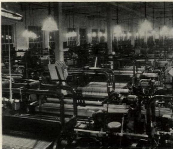
Silk mill. Weaving. 200-watt lamps, prismatic bowl reflectors. Outlets 6' centers in weaver's alley, 12' centers in rear alley. Lamps 9' above floor. Ceiling 13', ceiling white, walls white. Illumination level on work 25 foot-candles; on back of looms 6 foot-candles. Arohson Silk Mill, Coatesville, Pa.
