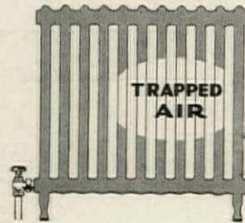
MANY contractors have experienced this trouble. When new water radiators are used on a steam job the steam short circuits across the top openings and closes the air valves before all the air has vented. This trapped air greatly reduces the heat output of the radiator—and often to such an extent that additional sections are necessary.
