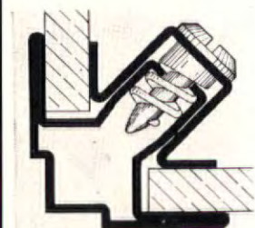
Sash B-1 and Corner Bar B-2 of "B" construction (Full Size). Sufficiently sturdy and graceful for the largest and finest store fronts.
