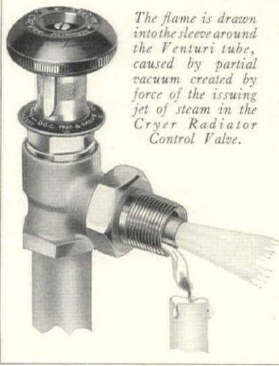
The flame is drawn into the sleeve around the Venturi tube, caused by partial vacuum created by force of the issuing jet of steam in the Cryer Radiator Control Valve.
