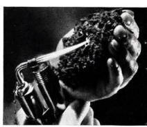
· Giving Eagle Home Insulation the fire test. Even when subjected to the flame of a blow torch, it does not char or burn. By filling hollow walls which ordinarily act as flues once a fire starts, Eagle Home Insulation provides real protection against the fire hazard.
