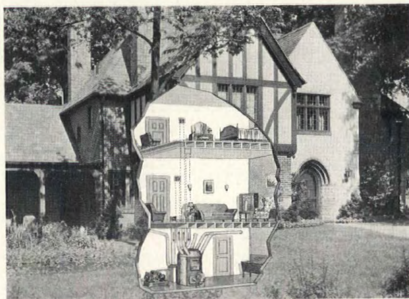
A combination warm and cool air system is shown in this picture. Details are given in the plan shown below.
