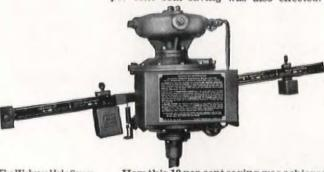
The Webster Hylo Steam Variator—a simple, rugged central control for use with Webster Systems where distribution of steam to all radiators is balanced by accurately sized metering orifices. The Hylo Variator Valve Operator (illustrated) automatically throttles a rugged motor-operated valve in the steam main.
