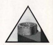
GAS ELIMINATOR Sucks gases out of coal tube and discharges them into firebox, where they are completely consumed. Consequently, the Whiting Hopper does not need to be airtight. The Gas Eliminator prevents back-firing and back-smoking.
