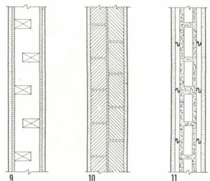
9. Staggered studs, 3-coat plaster on plaster board, sound reduction more than 50 db; 10. 8" brick, plastered: 55 db; 11. Hollow block, plaster on resilient furring; just under 60 db.
