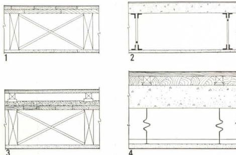
1. Regular wood joist construction, plaster ceiling, sound reduction 40 db; 2. Concrete supported by 8" open truss steel joists, plaster ceiling: 55db; 3. Regular wood joists, "floated" floor: 55 db; 4. Concrete slab, "floated" floor, resilient ceiling: 60 db.
