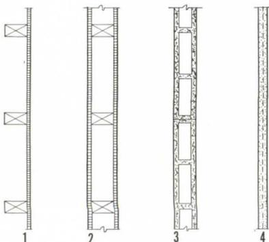
1.-2. Wood studs and wall board, unplastered, sound reduction 15 to 30 db; 3. Unplastered hollow block and light-weight masonry: 35 db; 4. Very thin solid plaster: less than 40 db.
