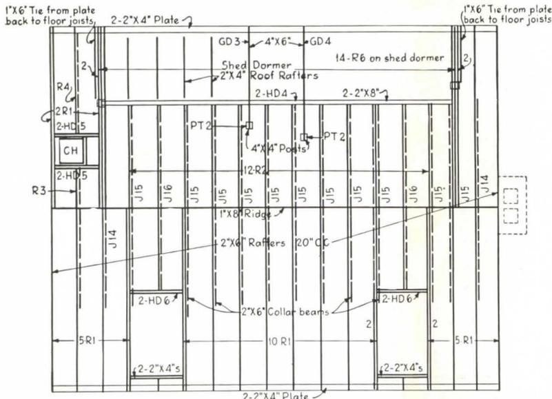
"Correct your mistakes on paper," says Builder Rausch. This roof framing plan was devised to indicate the number and type of framing members. On typewritten sheets the necessary members are detailed for each house, giving their code number for the framing plan, their size, number required.
