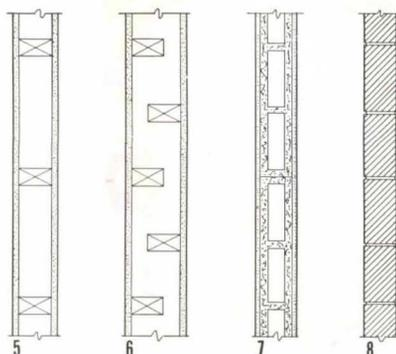
5. Wood studs, plaster on lath, sound reduction over 40 db; 6. Same with staggered studs: 45 db; 7. Hollow block, plastered: 45 db; 8. Brick, 4 in., unplastered: 45 db.
