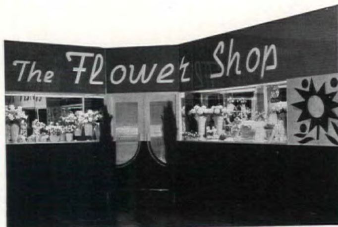
All-glass store front: sign, opaque and translucent "Vitrolux"—color-fused, tempered plate glass; decorated panels, "Vitrolite"; bulkhead black glass, sandblasted. Libbey-Owens-Ford Glass Co.
