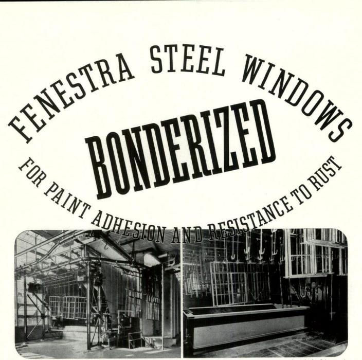
Fenestra Steel Windows emerging from the Bonderizing section in the new finishing building erected by the Detroit Steel Products Company
