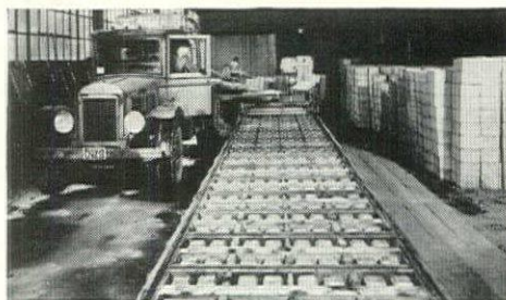
Manufacture of "Cemenstone" concrete blocks and other shapes proceeds with factory finesse. A pouring spout and vibrator ride atop a steel-framed mold (left). Vibration of the mix hastens setting, permits early removal of the forms, and thus continuous operation. Steam vats under the molds also contribute to production speed by stepping up the chemical reaction. When set, the blocks are removed for aging (right) which takes place under cover to keep quality constant.
