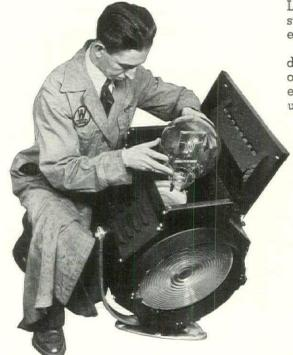
Westinghouse built the units required for the unusual lighting of the Perisphere. Incandescent fresnal lens projectors, as illustrated, were used in combination with multiple projectors, each using nine short-arc mercury lamps.
