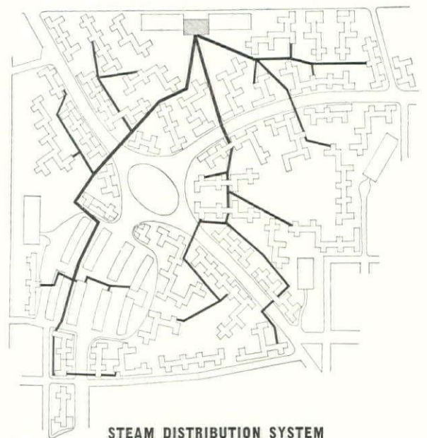
STEAM DISTRIBUTION SYSTEM
