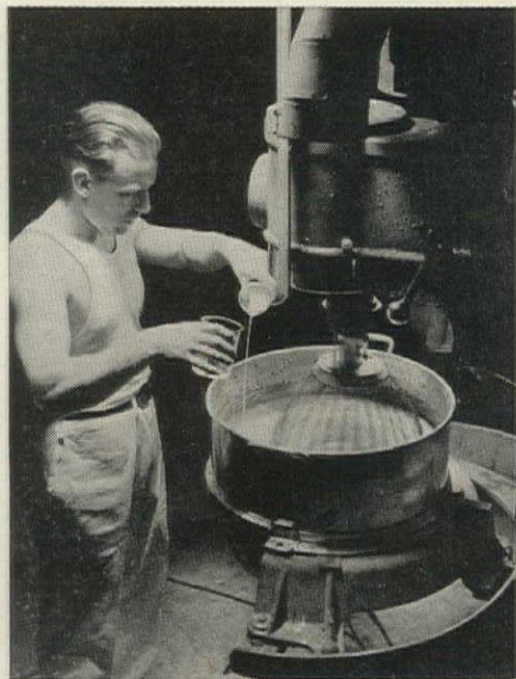
MANUFACTURE is by an entirely new process from liquid latex, the milk of the rubber tree, which is beaten into an air-filled froth, poured into molds, and baked. Upper pictures show native "milking" a tree, workman adding a jelling agent to beaten batch of latex, and operation of pouring an automobile seat cushion. Cores attached to the top of the mold form voids.
