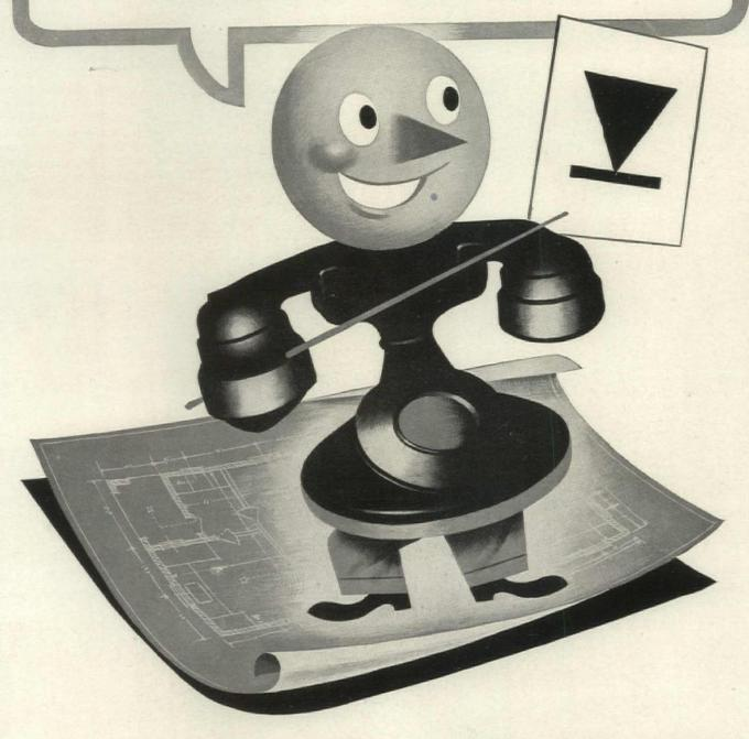
A SMALL TRIANGLE is the symbol you use to indicate a telephone outlet. This symbol, included in the plans you draw, is assurance that your clients will never have their walls and lovely woodwork marred by drill-holes and exposed wiring.
