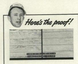
At the U. S. Forest Products Laboratory, Madison, Wis., these two sections of Douglas fir siding were painted exactly the same except for the first coat. On the left, the ordinary type of oil paint priming was used. On the right, an Aluminum first coat. Both sides then got the same two white topcoats. After 6 years exposure to sun and moisture, the Aluminum primed section was in far better condition as you can plainly see.
