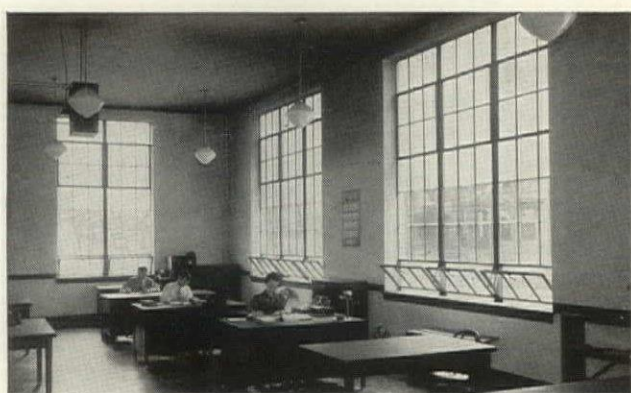
AKLO Hammered Glass is used in both the office and factory windows of the Druggist Cooperative Ice Cream Co., Inc., Atlanta, Ga.; Jiroud Jones & Co., General Contractor. In the office windows, only the upper half is glazed with AKLO Frosted Finish, permitting an unobstructed view through the lower half which is glazed with L-O-F Quality Glass. The factory windows are glazed throughout with AKLO.
