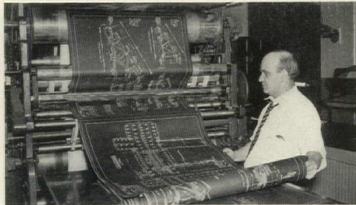
Blueprinting plans at rate of about 14 feet per minute
