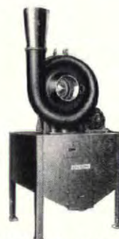
ROTO-CLONE TYPE "D" —for collecting process dust in dry form combines fan and dust collector in a single unit—eliminating expensive piping and high installation cost. Available in all sizes and capacities, also as self-contained unit including dust hopper and a filter to clean the exhaust air for recirculation into the workroom. Bulletin 272
